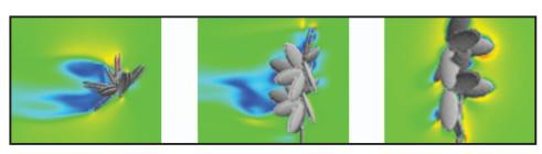
Simulation of flow around a mussel clump. Images courtesy of Blue Hill Hydraulics.
